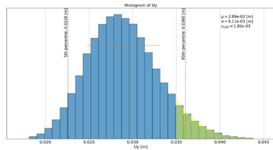
Correlations can be also taken into account. Here, introducing a negative correlation of -0.8 between c and  $\phi$  yields a new  $Pf(\text{settlement} > 3.5 \text{ cm}) = 5.2\%$ .
